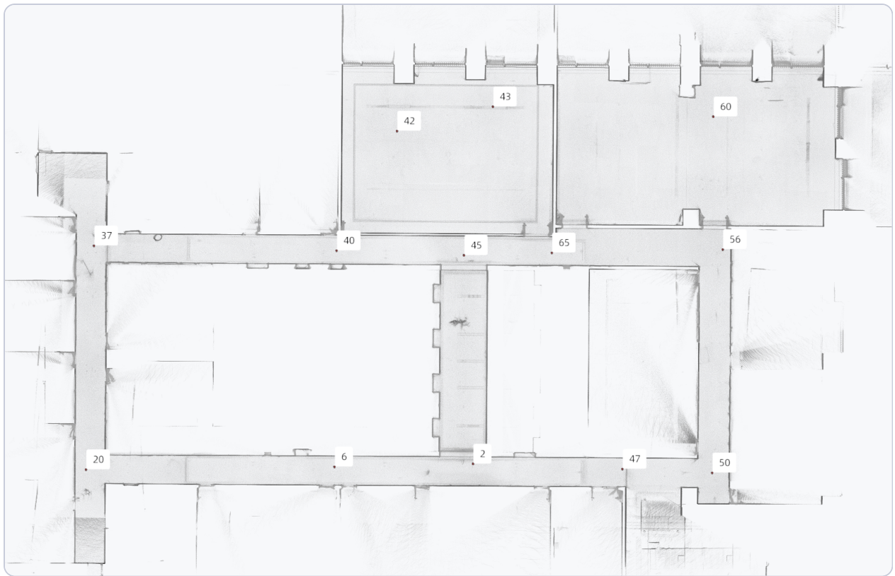
Figure 1: Top view of the test site point cloud and target distribution (the 13 targets included in the evaluation)
